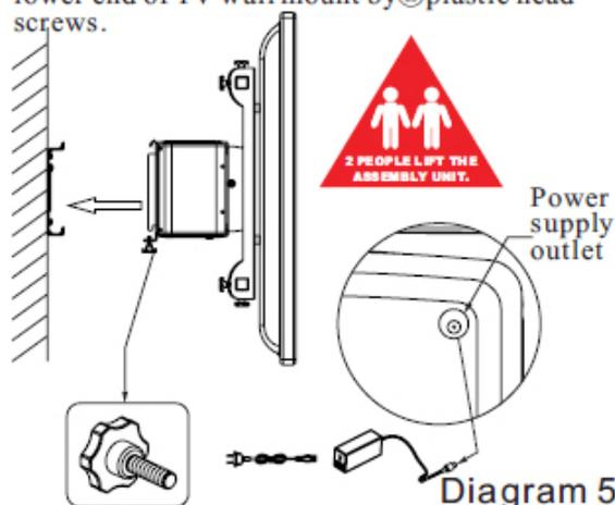
3-4. Hang TV wall mount (with TV) to the hooking gap of the mounting panel ,Then tighten the lower end of TV wall mount by (8) (2pcs) plastic head screws. (Diagram 5)
