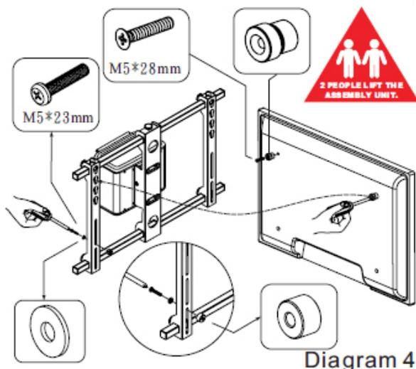
Hook TV wall mount (with TV) to the hooking gap of the mounting panel ,then tighten the lower end of TV wall mount by (8) plastic head screws.
