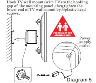
3-4. Hang TV wall mount (with TV) to the hooking gap of the mounting panel ,Then tighten the lower end of TV wall mount by (8) (2pcs) plastic head screws. (Diagram 5)
