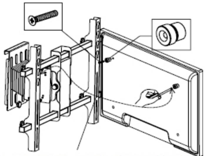
b: Hook TV by putting fastened hooking tabs into the corresponding holes on TV bracket.
