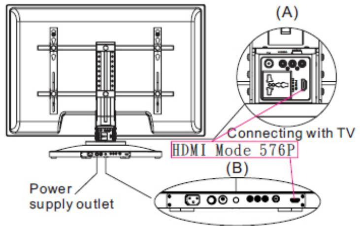
(Diagram 5) Connecting with external interface
