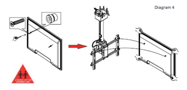
**3-5.** Through (4) washer and slot of TV bracket and (5) pad, (3) pan head screw fasten the down side of TV. (5) Pad should be placed between TV bracket and TV. (see the diagram 5)
