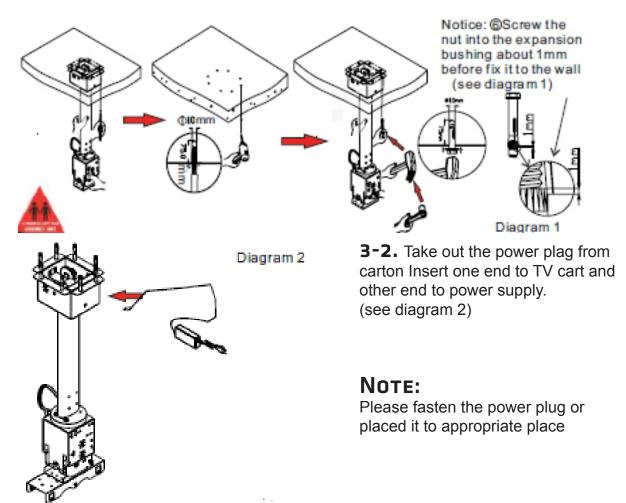
**3-3.** Connect power and press"Down"key on the remote control to let the cart pitch to horizontal position. Insert square tube into conjunctive bracket and fasten them by (7) round head screw. Hang TV bracket on square tube and fasten by (7) round head screw. (see diagram 3)
