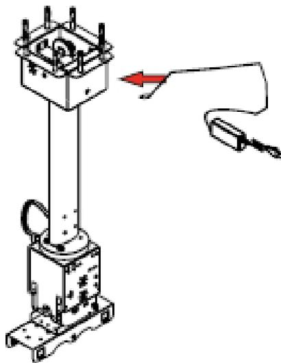
**3-2.** Take out the power plug from carton Insert one end to TV cart and other end to power supply. (see diagram 2)
